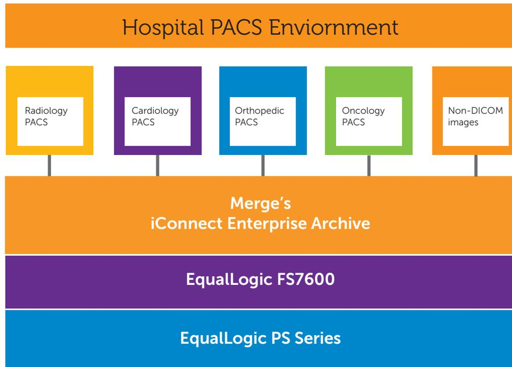
The above shows Merge's iConnect Enterprise Archive solution running atop Dell's EqualLogic FS7600 network-attached storage platform.
